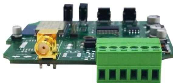
FIGURE 2: Antenna and green connector
