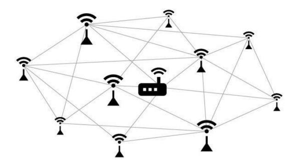
Mesh networks are also extremely reliable, since each device is connected to many other devices: if a node fails the network, due to hardware problems or any other reason, neighboring nodes simply look for other paths to transmit the signal (they turn to to other nodes). Network capabilities or resources can be increased simply by installing other devices.
